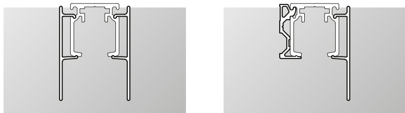
Valance profile - double sided mounting for ceiling mounted systems, single side mounting for wall mounted systems
